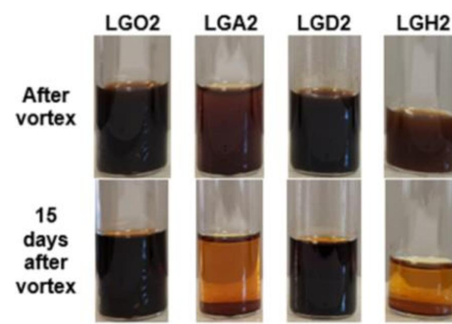
Sedimentation test of different types of lignin in the bioresin B=PEGDMA200/C10DA 50/50 [1]
