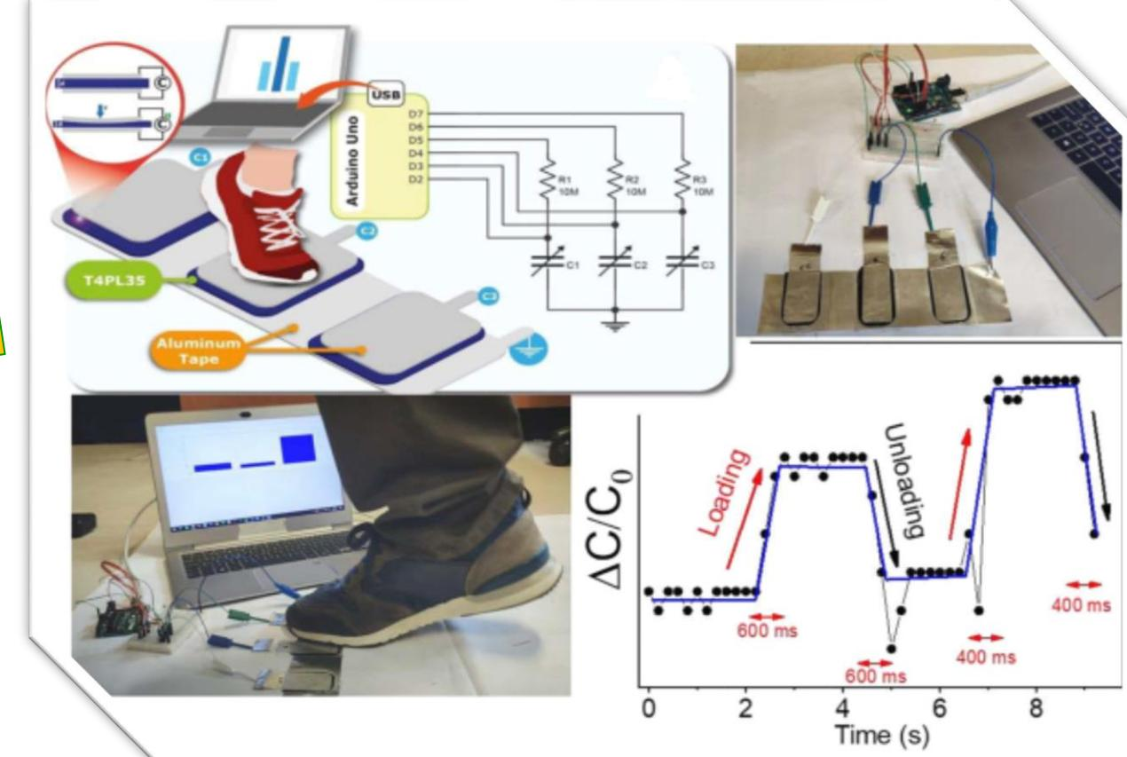
Proof of concept of a capacitive sensor developed with polyaniline-lignin as conductive filler. Reproduced from [3]
