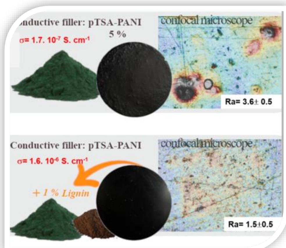
1 wt. % LGO improved dispersion, surface smoothness, ↑ wettability and ↑ electrical conductivity of 5 wt.% PANI-PTSA by one order of magnitude [2]
