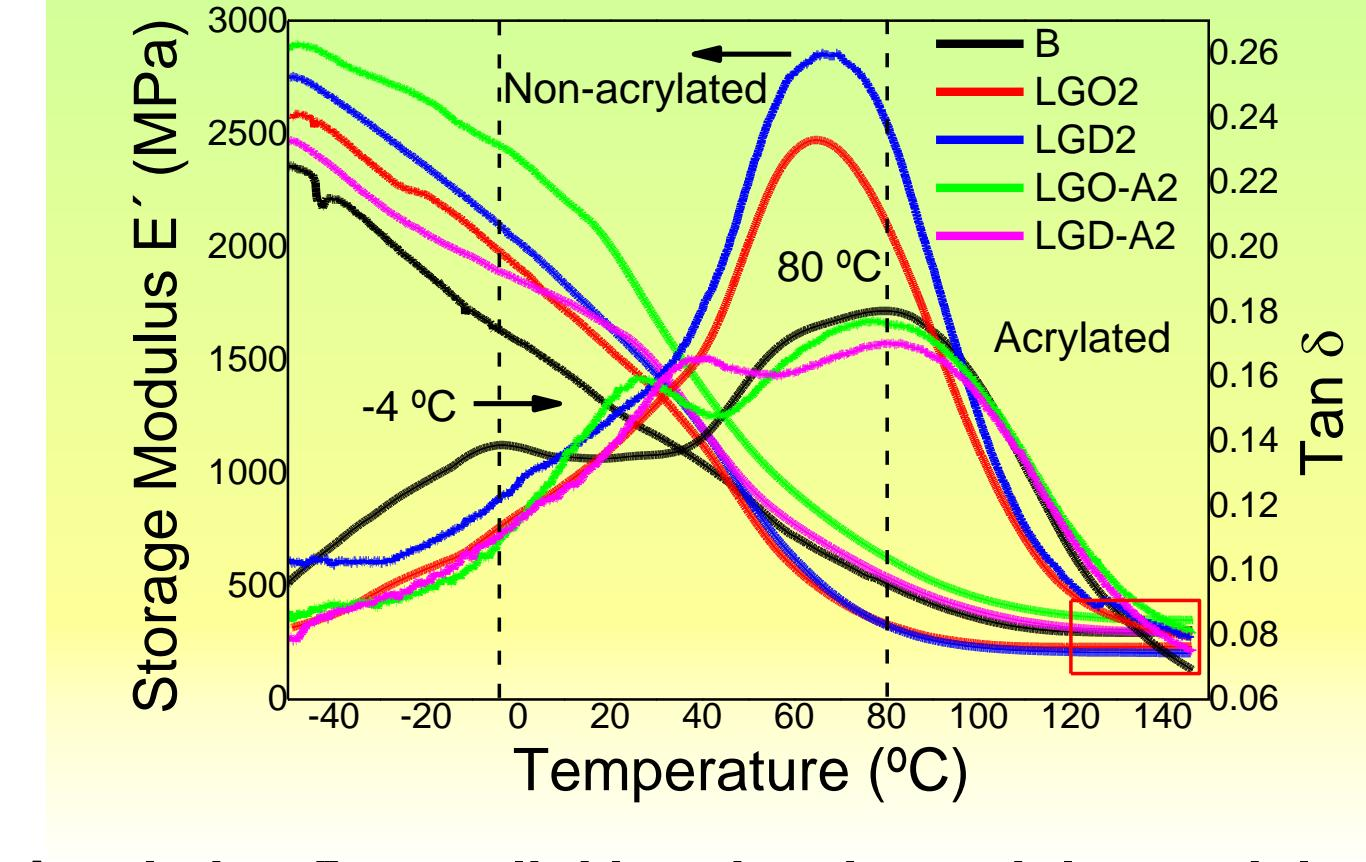
✓ Acrylation ↑ crosslinking density and the modulus above Tg. Non-acrylated lignin ↓ Tg.
