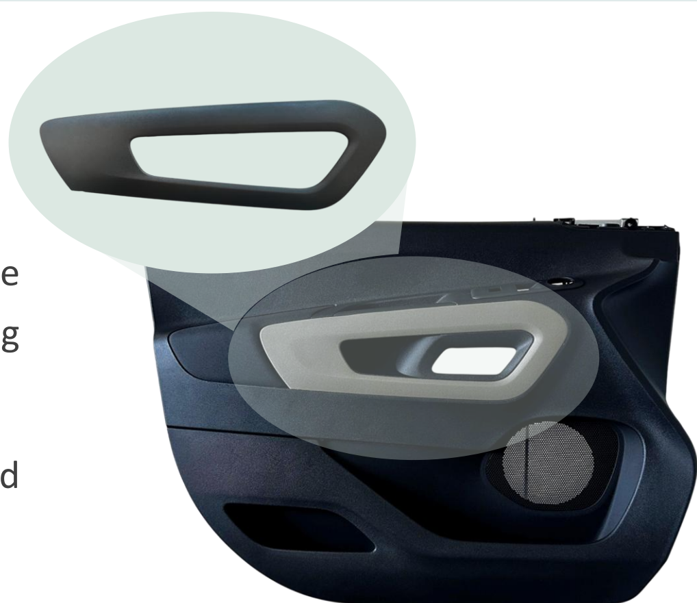
Injection-Moulded Automotive Component Based on PP/25Biopolymer/15UP Composite
