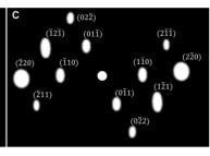
Coexistence of the [111] zonal diffraction of the DP phase (black dots) and the [110] zonal diffraction of the DD phase (orange dots)
