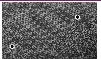
SEM micrograph of DG structure during slice and view, the holes correspond to the ion beam fiducials)
