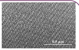
FIB cross sectional SEM image indicating the formation of network phase in a non-linear copolymer
