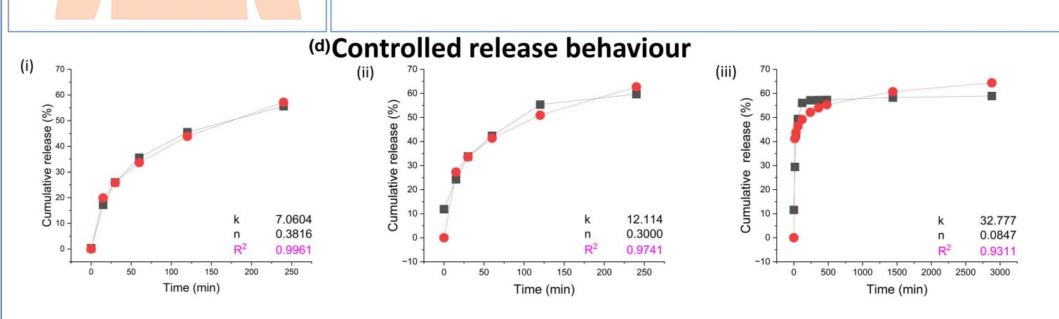
Figure 8. P 5 x 1.6 BAC sample undergo aggregation (a) in-vitro (b) Aggregation in Acid Orange 7 (c) simulate aggregation in-vivo and (d) Controlled release of differently charged dyes from P 5 x 1.6 BAC nanogel analysed using the Korsmeyer-Peppas model (i) Acid Orange 7 (negatively charge), (ii) Rhodamine B positively charge and (iii) Bromophenol Blue (neutral)
