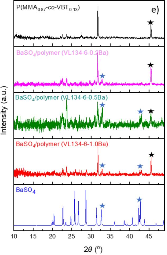
XRD patterns of barium sulfate, barium sulfate/polymer nanoparticles prepared with VBT units to BaCl<sub>2</sub> ratios
