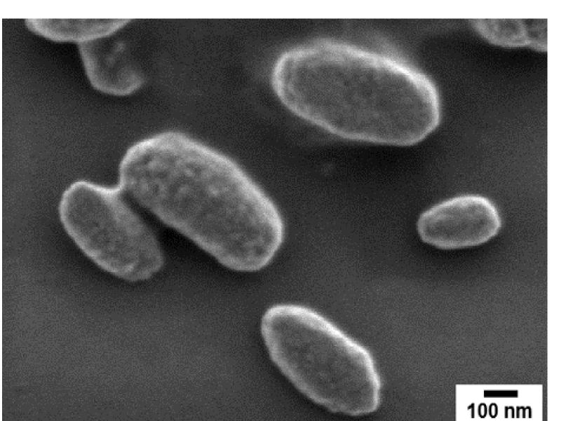
Micrograph of barium sulfate/polymer nanoparticles after filtration prepared with a molar ratio between VBT units and BaCl<sub>2</sub> of 2
