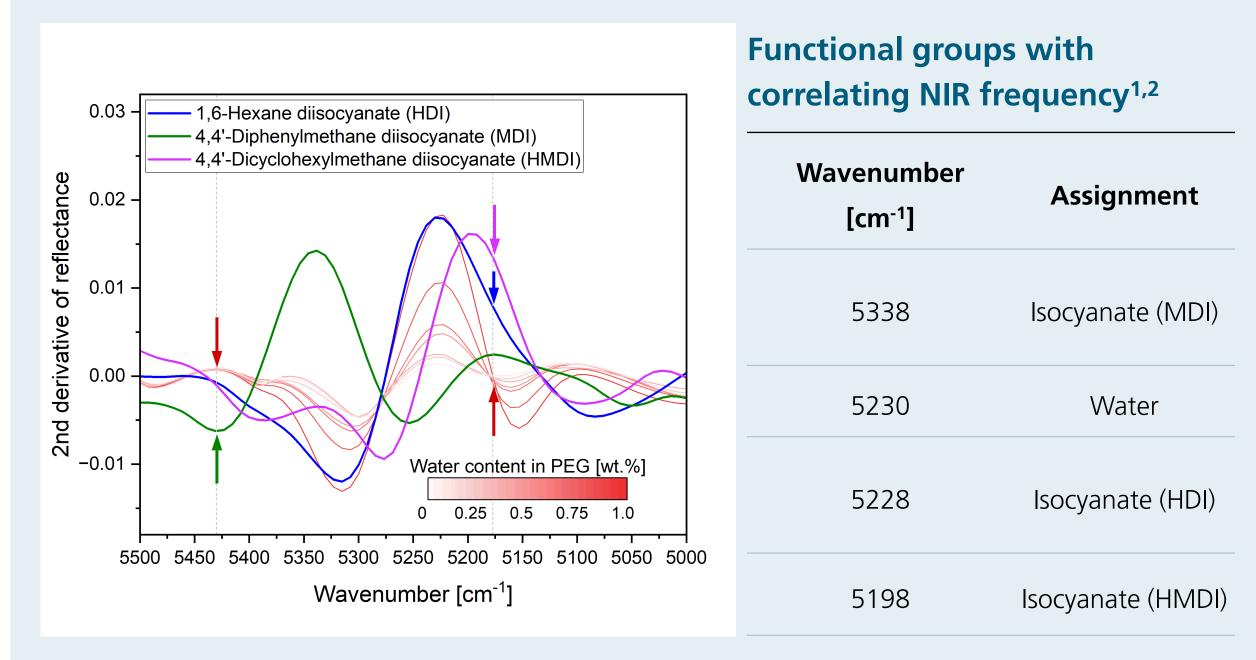
Derivative NIR spectra showing regions relevant for quantification of various isocyanates vs spectral range suitable for quantification of water in PEG
