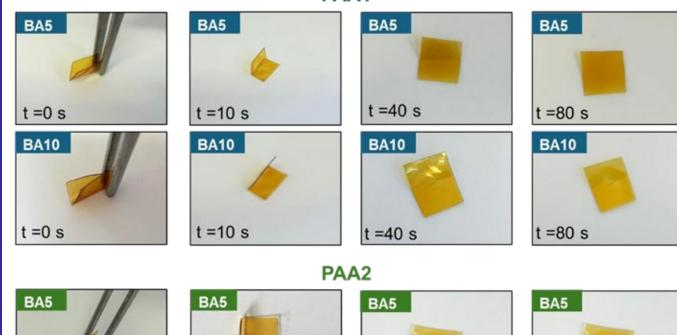
The images show a complete return to the original shape for both types of materials without external stimuli in less than two minutes
