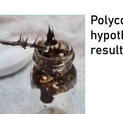
Solvent-free polycondensation at 120°C Self-condensation of the monomer
