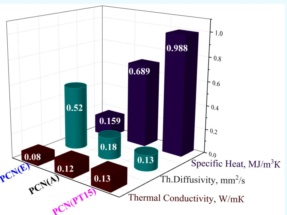
✓ All the PCN foams obtained exhibit low thermal conductivity values ranging from 0.08 to 0.13 W/m·K, indicating excellent thermal insulation performance.
