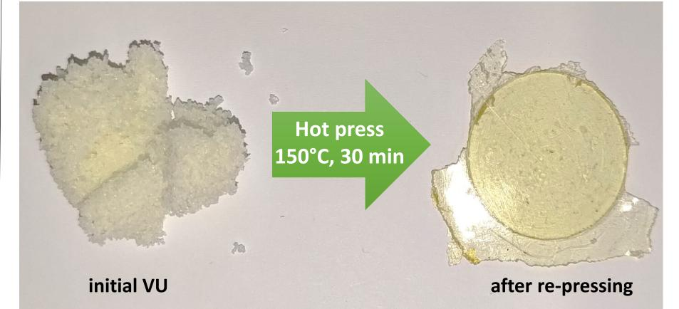
Re-pressed silicones do not exhibit any cracking
