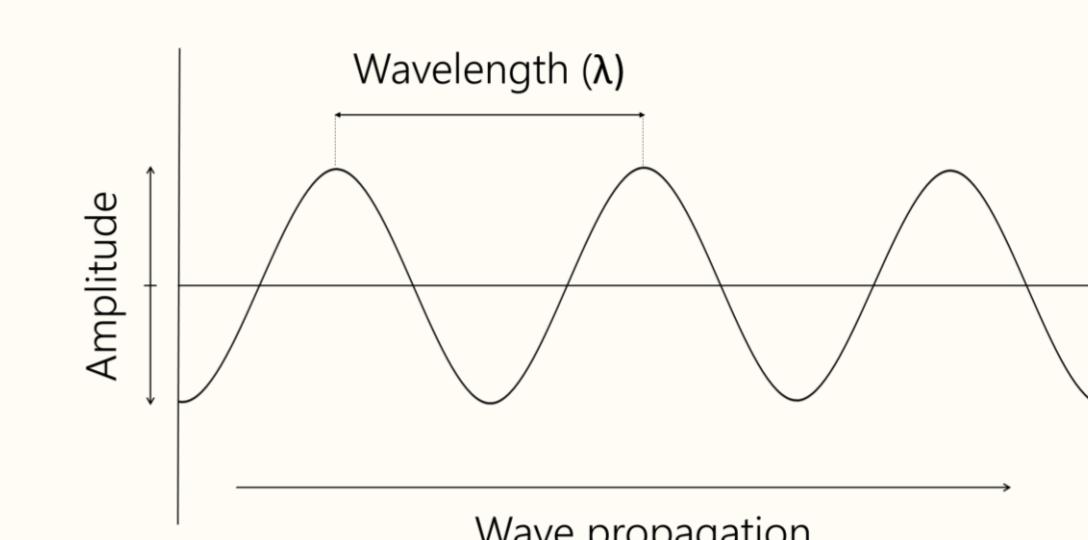
Ultrasound frequency range  $\geq 20$  kHz
