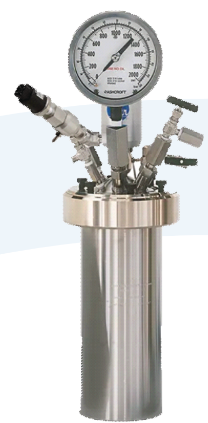
Fig 2. Parr 4570 autoclave used for Organosolv process.
