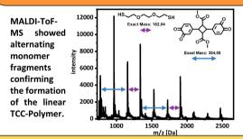
The sucessful TCC-formation was confirmed using 2D-NMR, FTIR and MALDI-ToF-MS.
