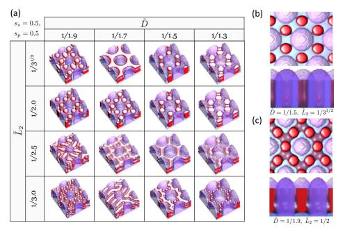
Effect of Surface Selectivity and Film Thickness on DSA (hexagonal array; B-selective substrate; B-selective pillar)
