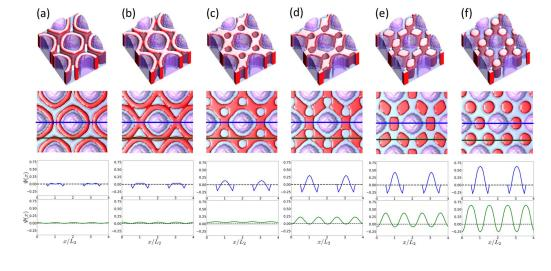
DSA Structure Map with Pillar and Substrate Selectivity (hexagonal array; B-selective substrate; B-selective pillar)
