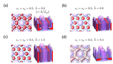
DSA Structure Map under Tetragonal Pillar Arrays (tetragonal array; neutral substrate; B-selective pillar)
