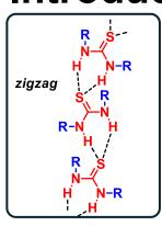
Incorporating hydrophobic domains into thiourea—ethylene glycol backbones enables robust, self-healing materials through flexible hydrogen bonding and domain formation. Unlike classical ureas, thioureas form more adaptable, zigzag H-bond arrays that support healing as demonstrated before by Aida et al <sup>1,2</sup>.
