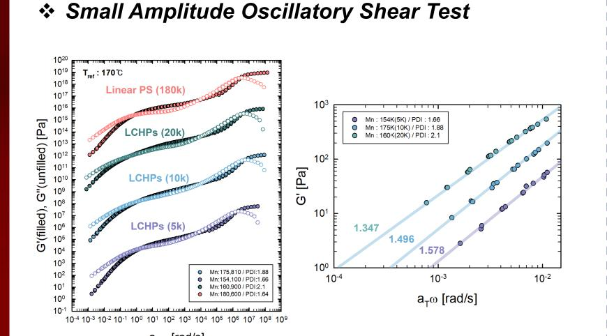
✓ As the branch length of LCHPs increases, enhanced entanglement leads to slower relaxation dynamics, evidenced by reduced terminal slopes and extended viscoelastic response. ✓ Longer branched structures exhibit enhanced strain hardening behavior, indicating that increased branch length leads to greater resistance to extensional flow due to more effective entanglement and molecular stretching.
