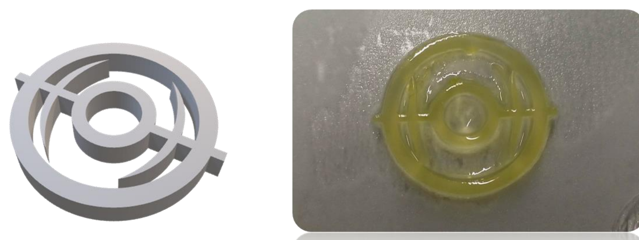
Fig. 3. CAD model and 3D-printed all-cellulose hydrogel using a DLP process
