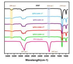
Near complete disappearance of the azide peak reflects the completion of the crosslinking
