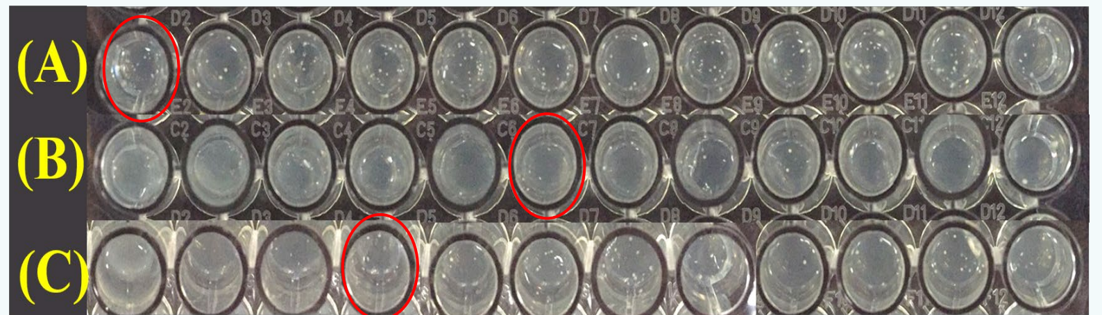
Fig. 7. Antibacterial activity of different fiber samples: (A) PEO fibers, (B) CS/PEO fibers at 15 mg/mL chitosan concentration, and (C) chitosan powder.
