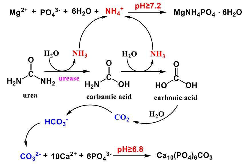
The mechanism of urease-catalyzed urea hydrolysis and formation of crystalline biofilm
