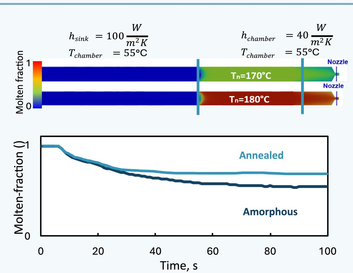
There is an interplay with the cooling rate, diffusion and crystallization. In case of slow cooling (higher extrusion ratio) although the crystallization is not too high but the diffusion at the interface induce the mechanical performance of the parts.
