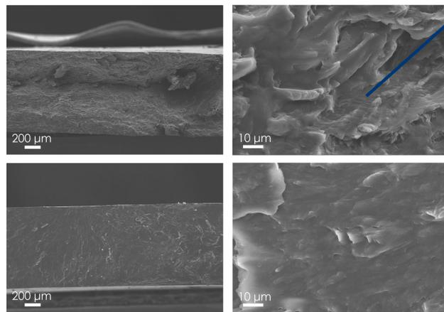
Textured surface due to fracture mechanism → **it breaks where there is a fibre**
