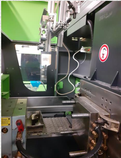
cartesian robot rides outside of mold space, injection overmolding starts
