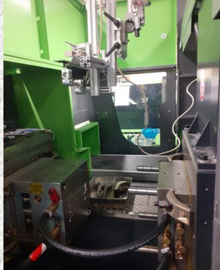
Quartz radiator mounted on cartesian robot gripper (stand by)
