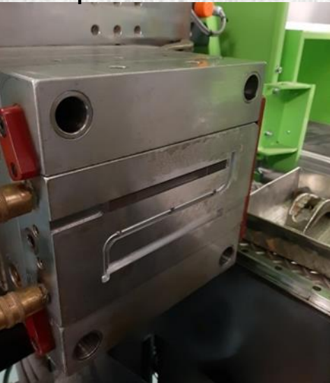
Insert emplaced in the cavity
