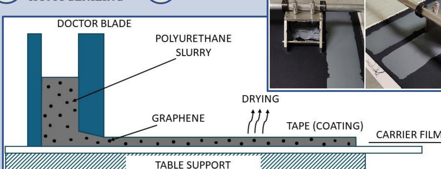
**CROSS-LINKING:** 1<sup>st</sup> heating: 120°C/15 min 2<sup>nd</sup> heating: 170°C/1 min
