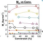
Polymerization conditions: : [IB]/[PC] = 2000/10; T= -30 °C; [IB]=1 M;  $CH_2CI_2/Hexane 80:20 v./v.$
