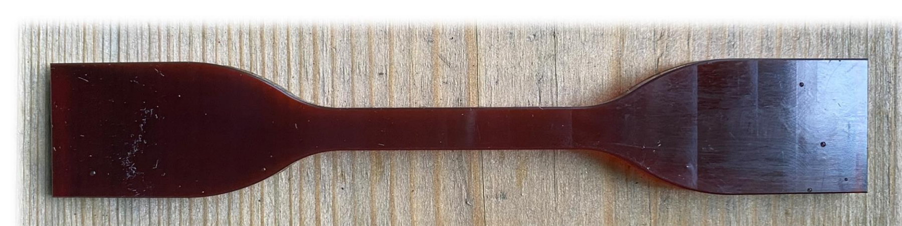
Figure 1. Cured dogbone-shaped specimen of resin 2.
