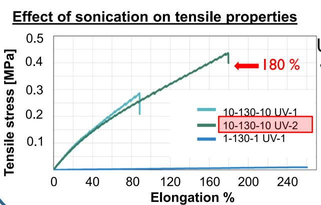
Ultrasound brings an energy boost, which leads to increased reactivity I. of BenEP units unsaturation => **f** ↑, **E** ↑
