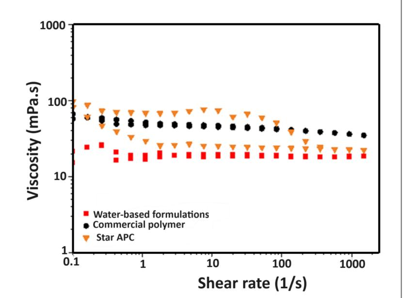
➤ star APCs - thickening comparable to commercial polymer at low shear, drop off at higher shear rates
