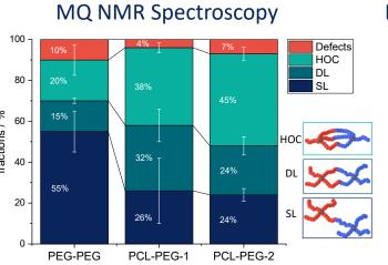
A comparison of the different connectivity fractions obtained for the various networks is presented. PEG-PEG was synthesized in  $D_2O$  according to the method of Sakai et~al. [1]. PCL-PEG-1 (R =  $NO_2$ ) was synthesized in toluene- $d_8$  according to the method of Bunk et~al. [2]. PCL-PEG-2 (R = H) was synthesized in toluene- $d_8$  according to our new method.
