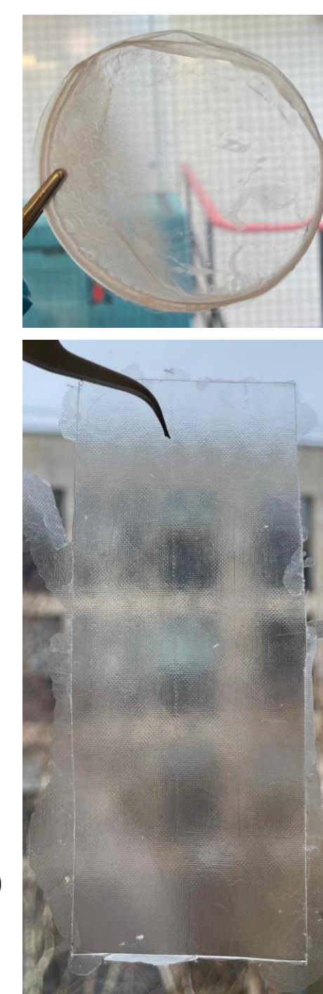
Figure 5: Copolymer films poly(LA-co-20 mol% CC): right; solvent cast from CHCl 3 , far right; thermal press (150 °C, 5 mins).
