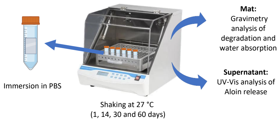
Fig 4. Scheme of the characterization of scaffolds immersed in PBS
