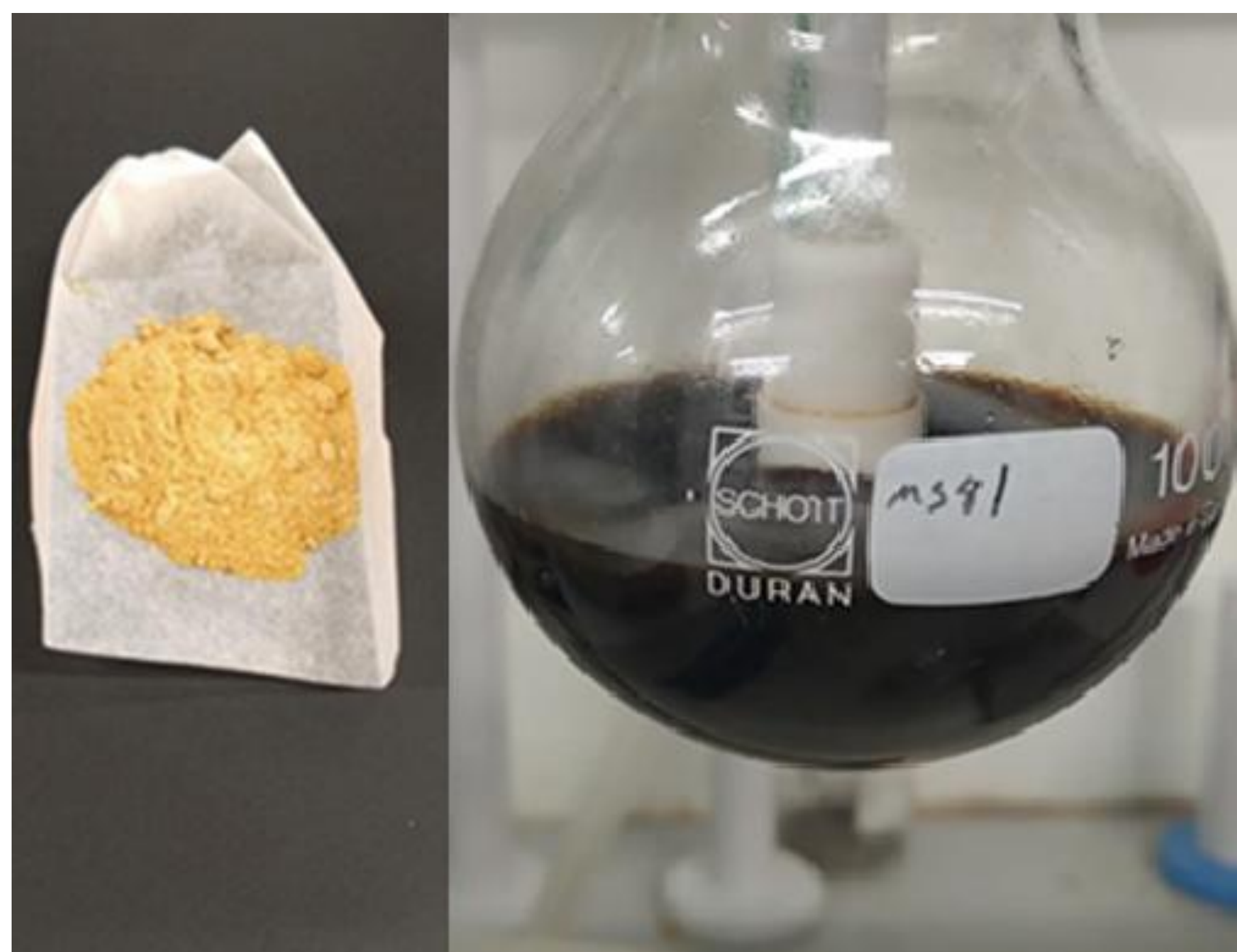
Figure 2. From bioderived monomer (left) to UPR ready for curing (right)
