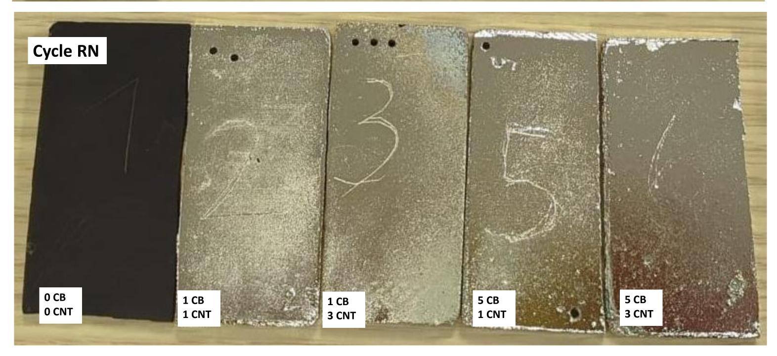
The coating was characterized using an Anton Paar microindenter, applying the Oliver and Pharr method to extract mechanical properties such as hardness and elastic modulus from the load-displacement curves. This approach enabled precise evaluation of the surface mechanical response of the plated layers.
