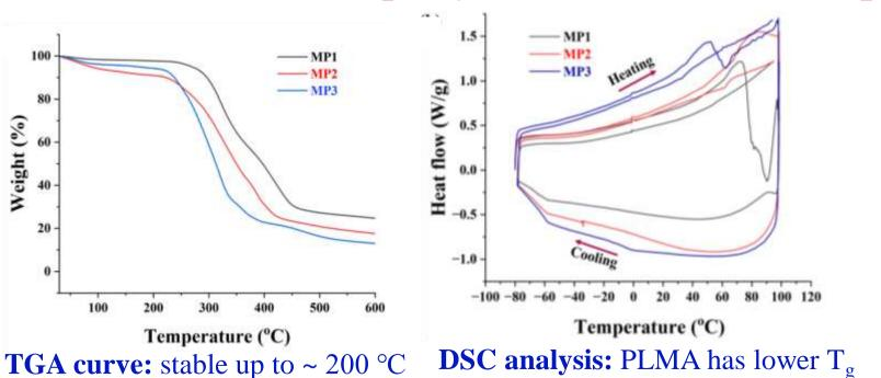
**DSC analysis:** PLMA has lower T<sub>o</sub> than PBMA and broad endothermic peak at higher temperature
