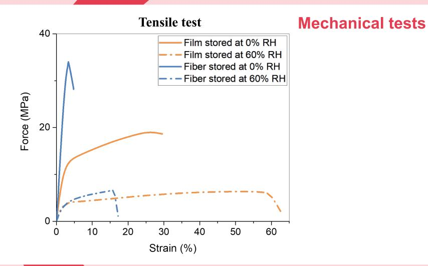
0% RH 60%RH Storage Young modulus (GPa) **HPC** fibers  $1346 \pm 148$  $258 \pm 76$ **HPC** films  $657 \pm 44$  $272 \pm 20$ **Tensile strength (MPa) HPC** fibers  $35.7 \pm 6.0$  $8.0 \pm 1.4$  $4.2 \pm 0.6$ HPC films 19.1 ± 1.1 Strain (%) **HPC** fibers  $18.4 \pm 5.3$  $3.5 \pm 0.7$
