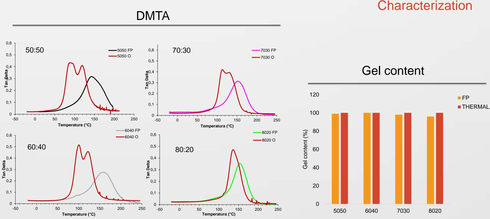
The glass transition of RICFP systems merely varies with the diluent content. However, in the epoxy:amine system, two peaks are observed, probably related to the existence of a double network.
