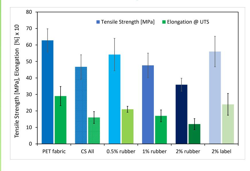
Tensile Strength & Strain
