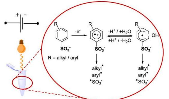
We aim to establish the major degradation pathway of proton-exchange membranes (PEMs). [2] To this end, we irradiated aqueous solutions of phenyl sulfonate-type model compounds with a Xe arc lamp, thus generating radicals. The radicals were trapped by DMPO, and the formed adducts were observed by EPR.
