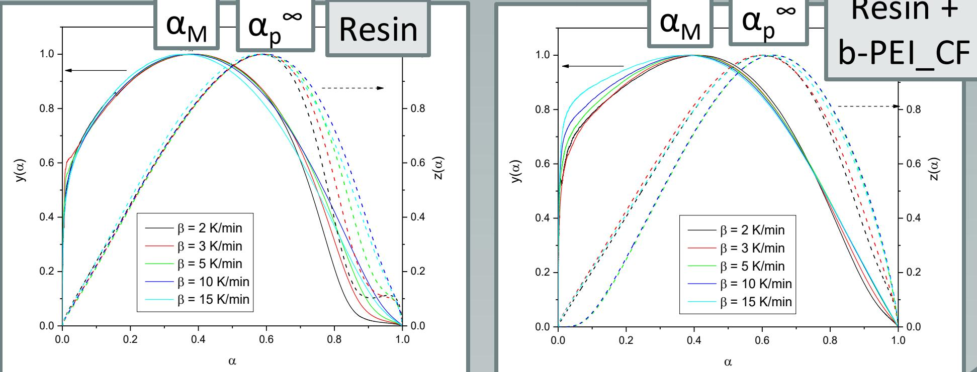
2 Kinetic equation applying the autocatalytic model
