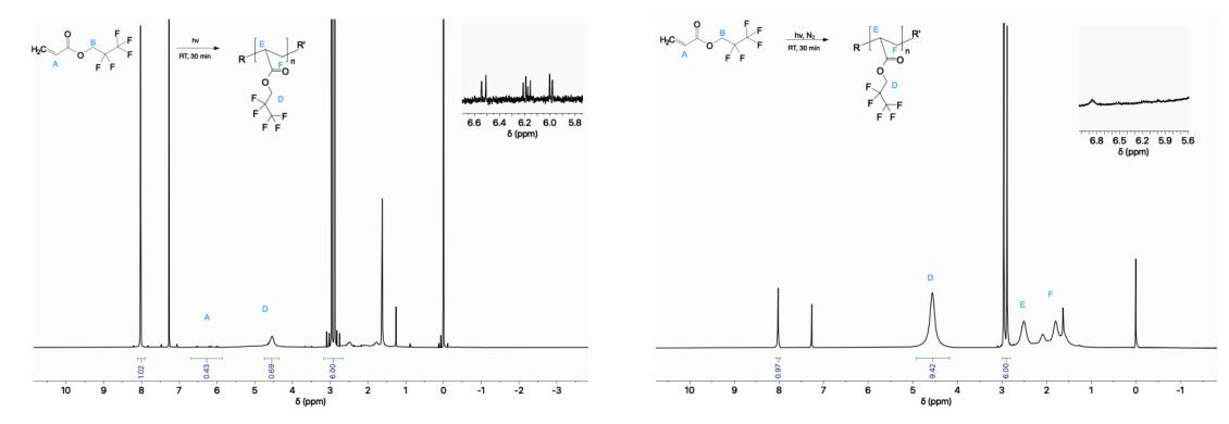
NMR analysis confirmed the impact of oxygen inhibition. Left - Polymerization without prior N<sub>2</sub> atmosphere: a reduced polymer backbone signal (D) and a clear peak corresponding to the unreacted monomer (A). Right - Same polymerization under N<sub>2</sub> atmosphere: a strong polymer backbone signal and no detectable monomer peak, indicating improved polymerization efficiency.
