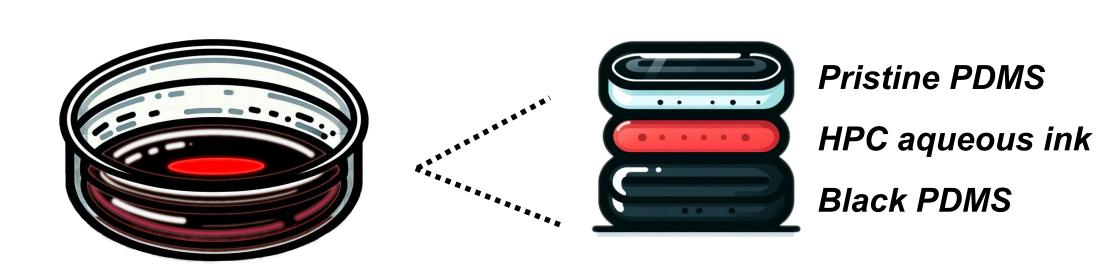
Mechanochromic sensor: The HPC aqueous ink was encapsulated and sealed between a black and a pristine PDMS layer.
