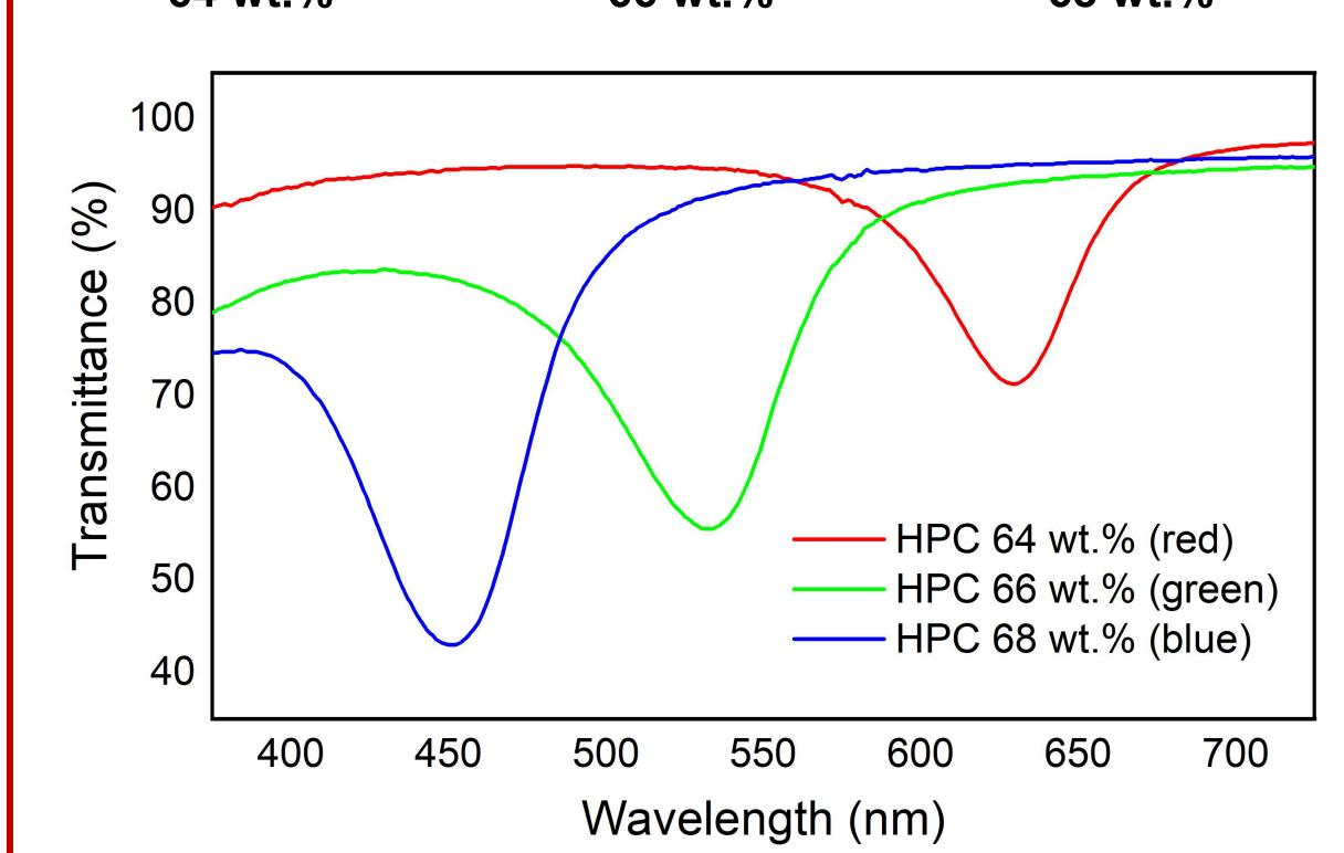
The mechanochromic sensors display striking structural colors that dynamically change under mechanical strain.
