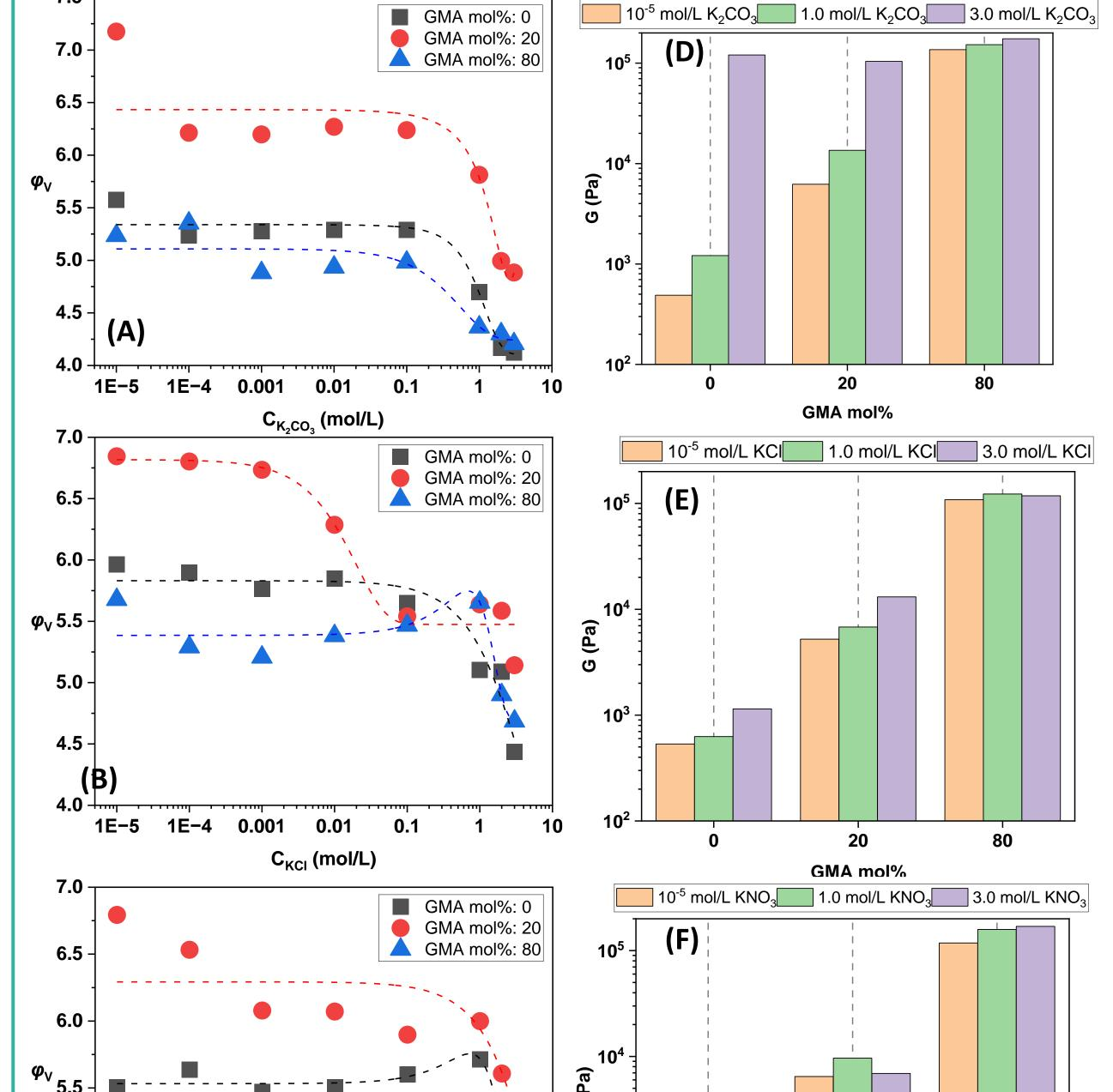
(A-C) Swelling ratio of PHm/Gn-XG gels at various GMA content after equilibrium swelling in aqueous solutions of K<sub>2</sub>CO<sub>3</sub>, KCl, and KNO<sub>3</sub>. (D-F) Swollen elastic modulus of PHm/Gn-XG gels at various GMA content after equilibrium swelling in same solutions.
