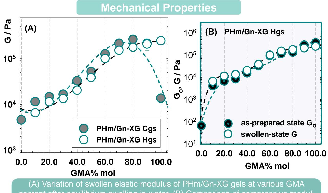
content after equilibrium swelling in water. (B) Comparison of compressive moduli of PHm/Gn-XG gels at various GMA concentration.
